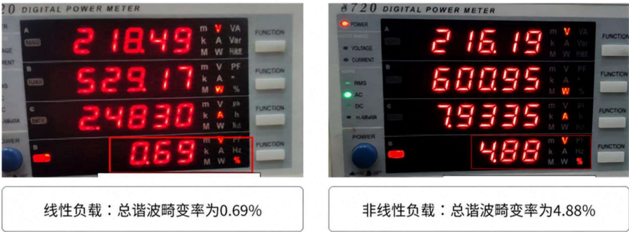
图 6 线性与非线性负载下输出电压 THD 实测 Figure 6 Measured Output-Voltage THD under Linear and Nonlinear Loads
