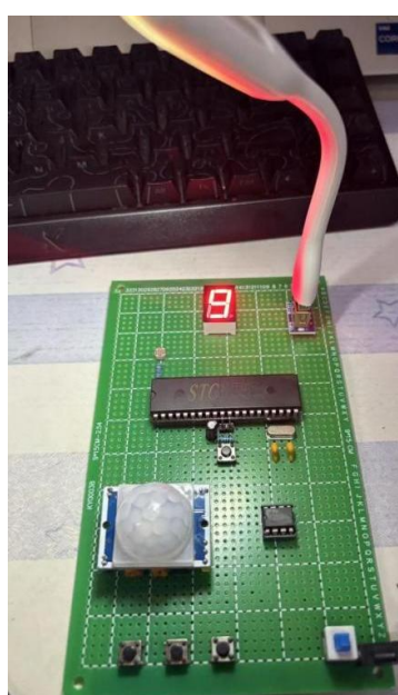
图 12 光照不足触发补光时系统状态 Figure 12 System Status When Supplemental Lighting Is Triggered under Insufficient Illumination
